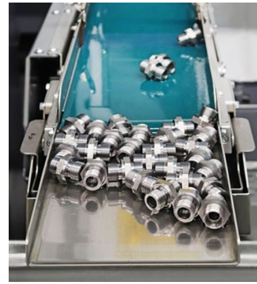
REA's latest investment: the new INDEX MS32-6 multi-spindle automatic lathe, designed for high productivity with short cycle times. REA produces 750,000 of these hexagon screw connections on this machine.
